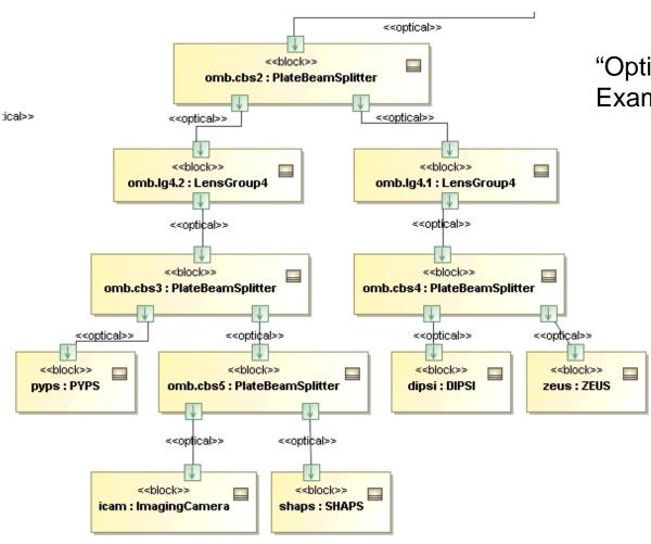
"Optical view" of APE: Example for using nested parts
