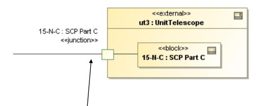
Use a junction port as a proxy for the internal block. Hiding nested blocks doesn't effect the relationships.
