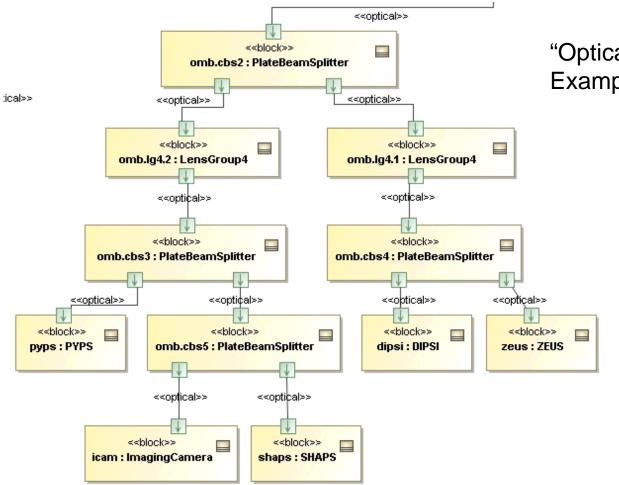
"Optical view" of APE: Example for using nested parts
