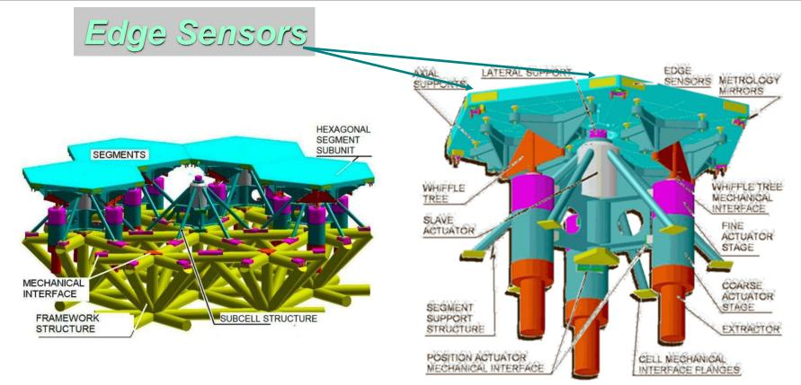
Detect nanometers of phasing error in micrometers of turbulence with Phasing Wave Front Sensors (~20 nm RMS)
