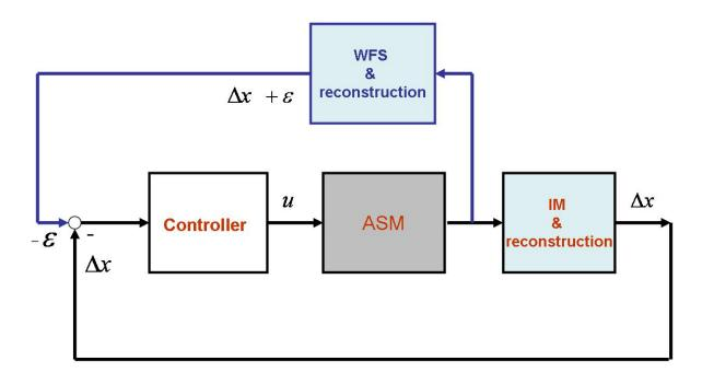
The control of the ASM has a cascade structure with two loops.
