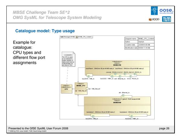
Different use of parts in different contexts (different items flow over the same type of connector). Here a 96 pin connector has a different assignment.
