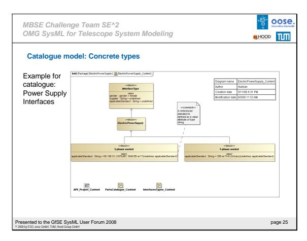
Catalogues can be easily extended by using inheritance. Furthermore the preliminary design of a system can work with an abstract type (when the detailed requirements are yet unknown) and decide later which specific type to use for the implementation.
