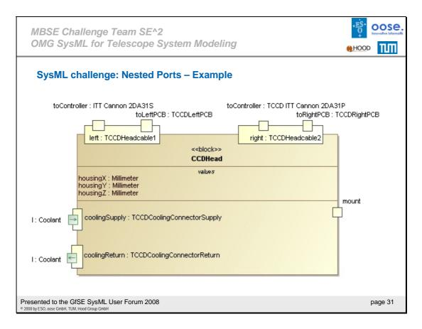
By using nested ports, the cable is a standard port with standard sub ports which represent both ends of the cable. This is particular useful when a cable is permanently soldered to a chip, like here to a CCD head PCB.
