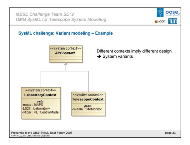
APE has two variants, represented by different contexts (Lab and Telescope). Depending on the context different parts must be used which are deeply nested in the product tree (e.g. Support structure in the lab and support structure on the telescope). The problem is how to relate this information, i.e. how do you model that those parts are depending on the context? Tags are used to associate parts with variants.
