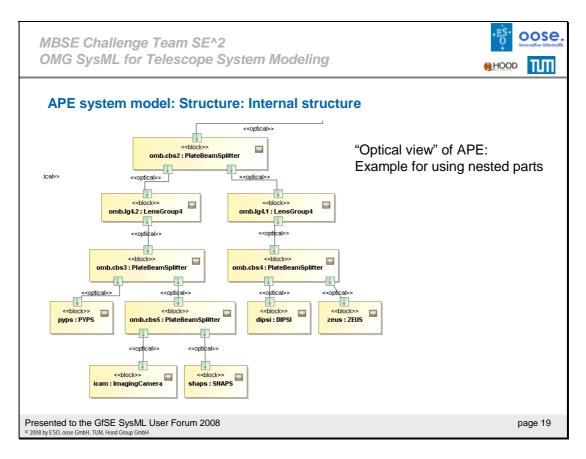
A model is much more than just a couple of diagrams. A model consists of multiple views showing different aspects of the system that are interconnected.
