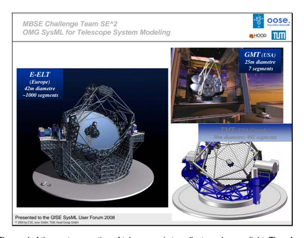
The goal of the next generation of telescopes is to collect much more light. Therefore very big mirrors are required which cannot be made any longer of one single piece. The drawing shows a draft of the mechanical structure of the European Extremely Large Telescope (E-ELT) and its competitors, the GMT and TMT. The E-ELLT will be about 70m wide, where the primary mirror is 42m in diameter.
