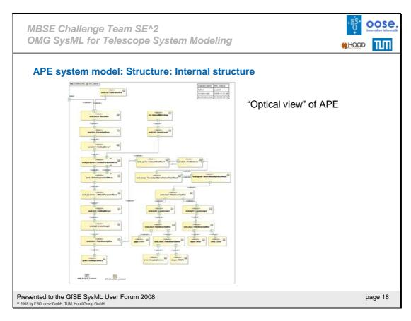
A model is much more than just a couple of diagrams. A model consists of multiple views showing different aspects of the system that are interconnected. The same components can be connected in different views in different ways. This diagrams shows the optical layout in an abstract manner.
