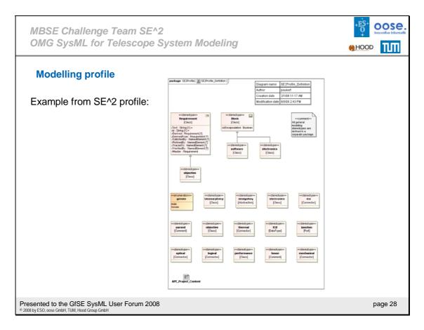
The SE^2 profile extends the SysML by adding stereotypes for different connectors (optical, mechanical), specific block types (Software, Electronics).
