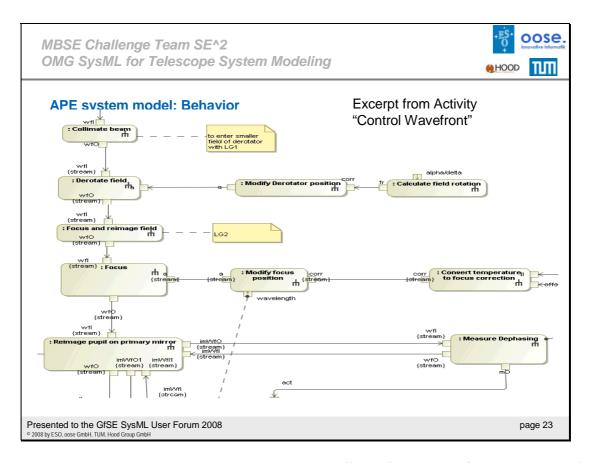
The model shows at the same time the physical effect of a system (like distortion of wave front) as well as sensing, actuating actions and control flows.
