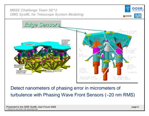
The wave front is distorted by various factors: one of them is a wrong positioning of the segments of the primary mirror which will result in a discontinuous surface. This is compensated by the so-called phasing loop.
